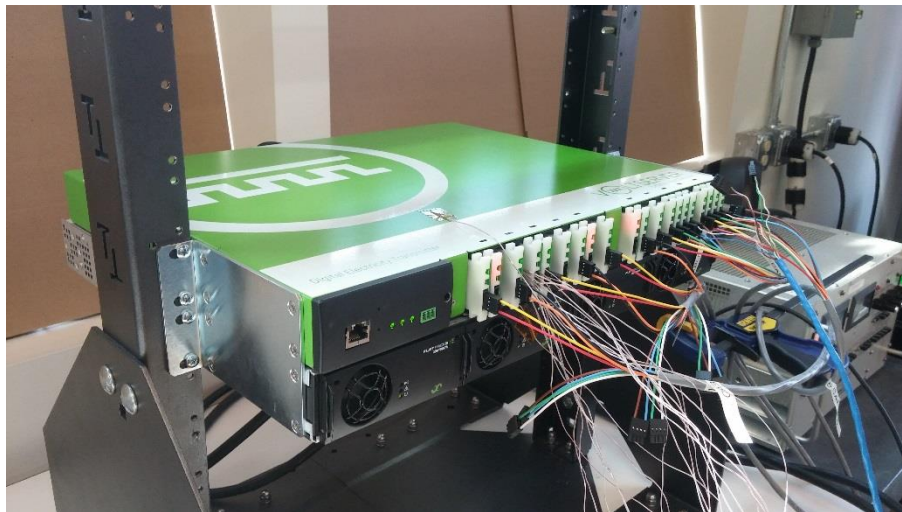
Figure 7: VTX500 Instrumented for Thermal Testing
