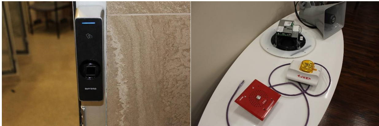
Figure 5-5: POE access control (left) and assortment of POE safety/ communication devices (right)
