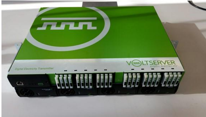
Figure 6: Completed VTX500 12kW Transmitter Unit
