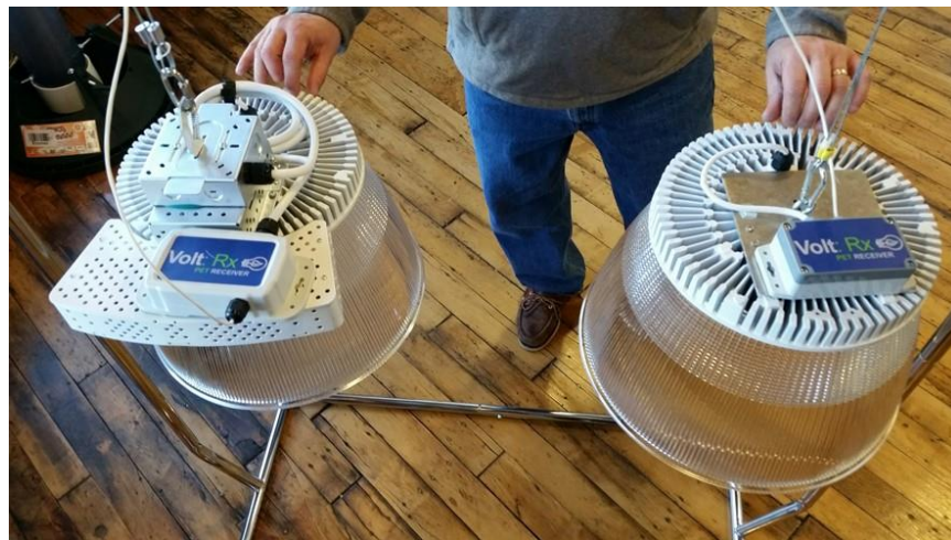
Figure 3: Cree Dual AC/DC High-bay (left) and Direct DC Drive (right)
