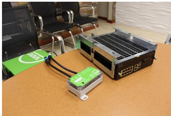
Figure 6: VoltServer RX520 receiver with Cisco CDB PoE switch
