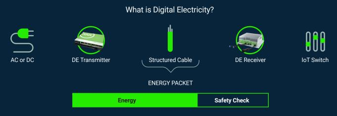
Discrete "packets" of electricity. Each checked for safe transfer from transmitter to receiver. 500 safety checks per second.
